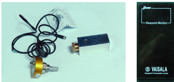
Picture 6-6: Parts of Dew-point Monitor
