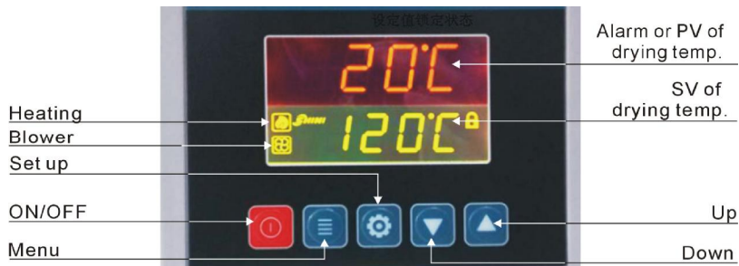
Picture 4-1: Control Panel
