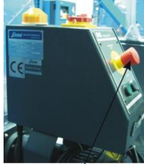
Emergency stop button
