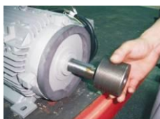
Picture 3-15: Installation of Belt and Belt Pulley 5
