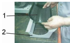
Picture 3-22: Installation of Screen and Screen Frame 1
