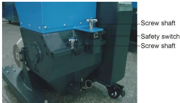
Picture 2-4: Safety System
