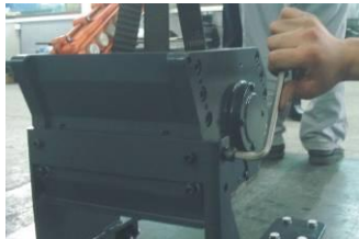
Picture 3-11: Installation of Belt and Belt Pulley 1
