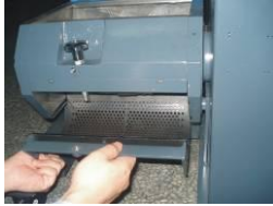
Picture 3-23: Installation of Screen and Screen Frame 2
