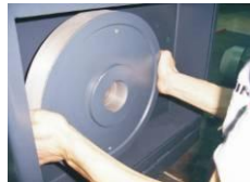
Picture 3-12: Installation of Belt and Belt Pulley 2
