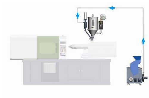
Picture 2-39: Loading With Blower
