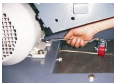
Picture 3-19: Installation of Belt and Belt Pulley 9
