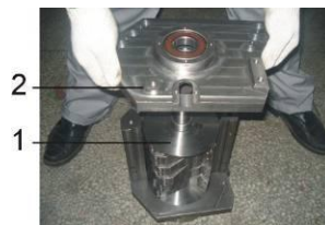
Picture 3-5: Installation of Bearing and Blade Rest 3
