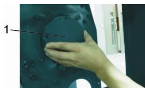
Picture 3-6: Installation of Bearing and Blade Rest 4
