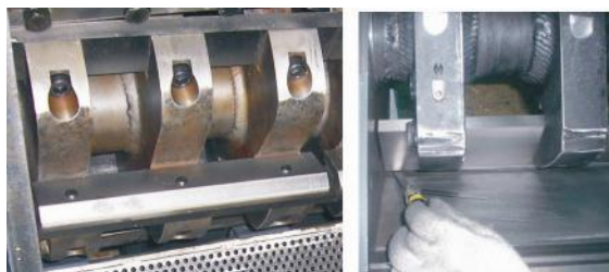
Picture 3-4: Installation of Fixed Blades and Rotating Blades
