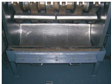
Picture 4-3: Close the screen bracket; the regrind storage bin and the feeding hopper
