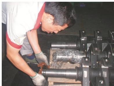
Picture 6-5: Installation of Bearing and Blade Rest
