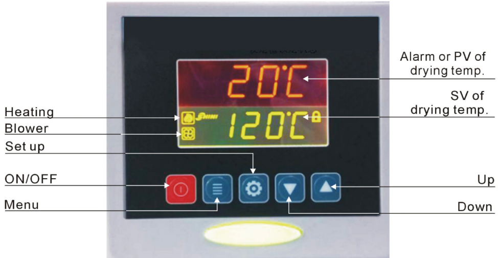
Picture 4-1: Control Panel
